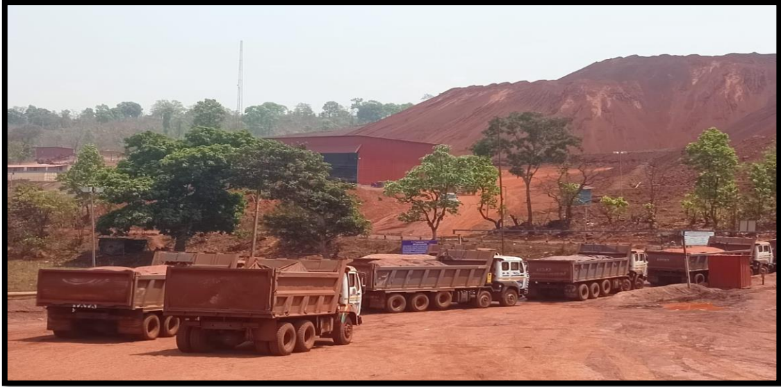
Photo #7 Ore Carrying Vehicle covered with tarpaulin before exit of mine gate
